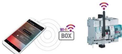
In order to prevent an "out of service" of the Wi-Fi box in case of remote/local command or in case of tripping due to failure, the power of Wi-Fi-box should be taken from a different line from the one on which you installed the Stop & Go or, in the case it is not possible, we recommend to backup the Wi-Fi box via UPS.
